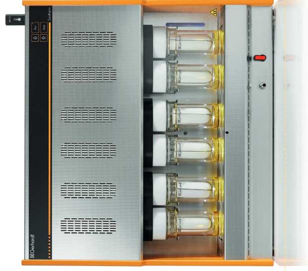
Stage 2: Solvent reduction, collection of distillate
