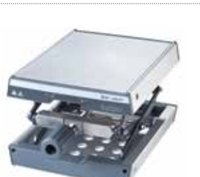
LABLIFT m Laboratory lifts lift and support small pieces of laboratory equipment and containers. A maximum weight of 7 kg (maximum dynamic load) can be lifted. Carrying weight: up to 25 kg (max load). The working height is between 70 mm and 300 mm Ident-No.: 0004022400
